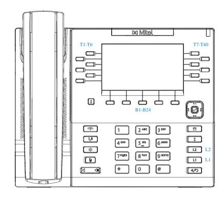
The Mitel 6869 consists of handset, screen, navigation/select key, numpad, option keys, line keys (L-keys) and softkeys (T-keys and B-keys).
